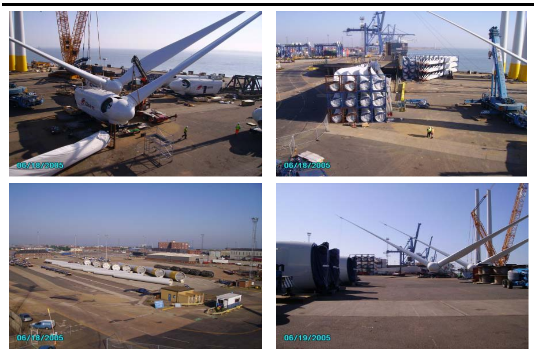
Box 1 Images taken from a typical laydown area for onshore assembly of wind turbine components
